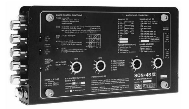
The essential information for connecting to and operating the mixer is permanently printed on the baseplate.
